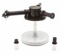
by means of the reflection on a face of the prism. The equilateral prism made of highly dispersive material. With this device you can study the spectrum of a source of monochromatic or polychromatic light. We recommend the use of interferential filters to the check of the wavelength.
